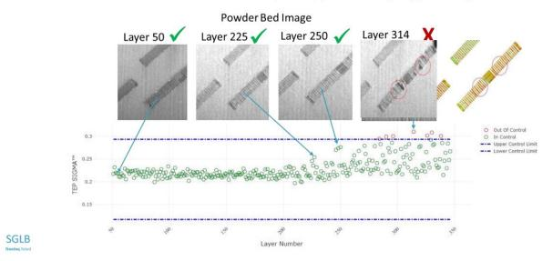
We think the sample above is relatively straightforward. In this case the manufacturer set QA thresholds that it determined to be acceptable QA metrics (the "upper and lower control limits"). Notice as the layering proceeds and gets beyond layer 225, the consistency begins to drift to the upper boundary of the acceptable control limit. As the process progresses into layers 300 and beyond, one can see that the process is trending towards the upper
